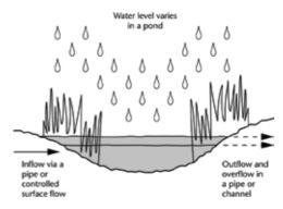
The level of solids removal can be significant when enough time for detention is allowed. The algae and plants of wetlands provide a particularly good level of filtering and nutrient removal. Ponds and wetlands can be fed by swales, filter drains or piped systems, and the use of silt traps will help to manage sedimentation.
