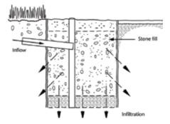
with a perforated pipe which carries flow along the trench. This enables the storage, filtering and some infiltration of water passing from the source to the discharge point. Pollutants are removed by absorption, filtering and microbial decomposition in the surrounding soil. Systems can be designed to successfully incorporate both infiltration and filter systems.
